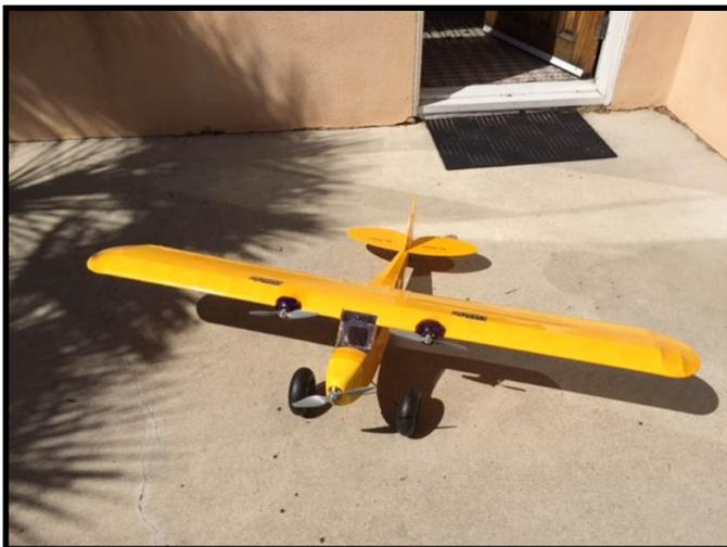
The plane came in at 2.4 lbs. - quite a bit under the stock 3.2 lb. target - and had over 325 watts of power with a fresh battery, so getting into the air was no problem. After the exciting first flight, all three motors were shimmed down with washers, and 5% down elevator was mixed with the throttle to gain level flight at all throttle settings. Flying is
