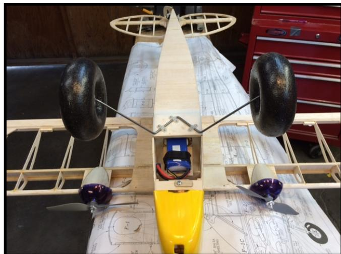
The bottom of the plane allows access to the battery and hatch cover. The 3S-2200ma battery is still in front of the CG by several cm, which allows easy adjustment of the CG.
