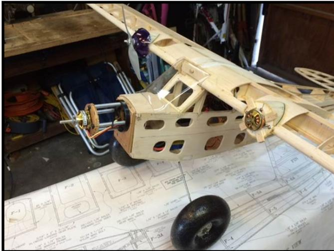
*With the cowls removed you can see the motor mounts.*
