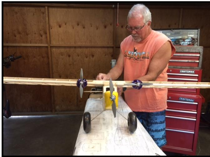
This plane is based on the Great Planes Electric Cub kit, circa 2000. The nearly complete tri-plane wing is being assembled by the handsome owner. Without the front motor, the battery would have to protrude out the front of the cowl to achieve the correct center of gravity. Note the tundra wheels - another engineering change implemented due to the owner’s apparent lack of ability to land on the infield. This is a relatively large plane for a park flyer, with a 59-in wingspan.
