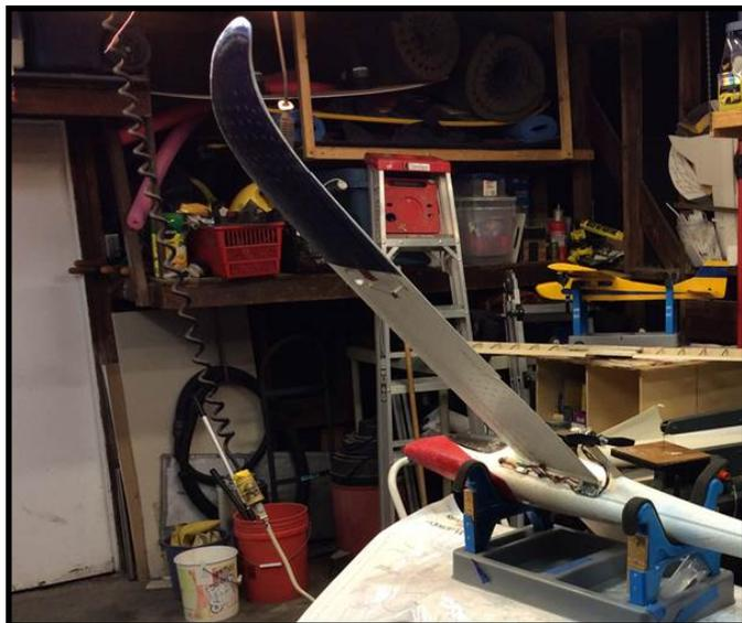
The ESCs are attached to the fuselage under the wing. No room for them under the canopy. To achieve the correct CG a large 3S-2200maH battery is pushed all the way forward in the nose. Flight times with that battery and modest power are about 25 minutes.
