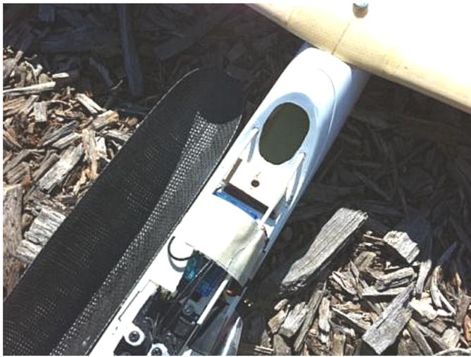
Ballast bar mount & opening in fuselage with 5 X 2.5oz. slugs
