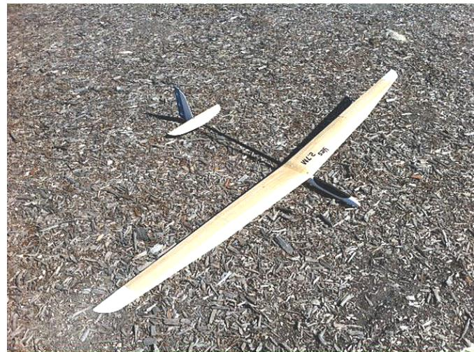
106" span, high-aspect-ratio wing and SD 7080 airfoil
