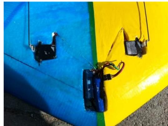
7) Attach the control linkage to servos and elevons.
