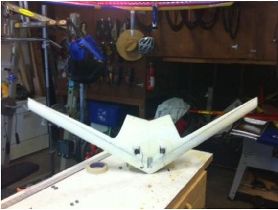
3) Next we replace the rear sections of the wing with balsa ribs and trailing edges. Carbon fiber tow is CA'd to the bottom of the trailing edge to improve structural strength. I notched the foam section to accept the balsa ribs and attached them using ZAP. I angled the ribs near the wing tips up a couple of degrees to add a little washout and minimize tip stalling.
